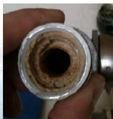
Conductor condition after three months of operation without and with AquaKat.
