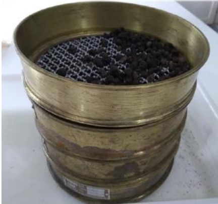
Figure 2: Screen set used for separating sheep manure fractions according to particle size (8, 4, 2 and 1mm).
